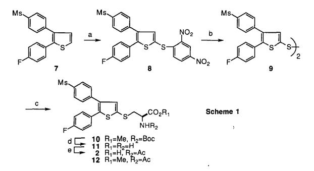
*Reagents and Conditions* : a, 2,4-(NO<sub>2</sub>)<sub>2</sub>C<sub>6</sub>H<sub>3</sub>SCl, TFA, reflux, 75%; b, aq. NaOH, MeOH, reflux then I<sub>2</sub>, MeOH, 67%; c, Boc-L-Ser-OMe, <sup>n</sup>Bu<sub>3</sub>P, THF, room temperature, 68%; d, 4N-HCl, AcOH, 100 °C, 65%; e, Ac<sub>2</sub>O, Et<sub>3</sub>N, Et<sub>2</sub>O, H<sub>2</sub>O, 0 °C, 91%.
